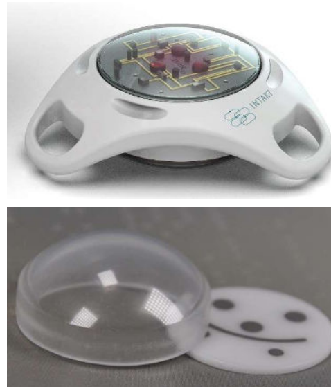
Active microimplant with housing made of spinel
